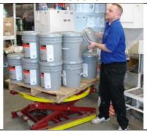
Positioner reduces bending associated with lifting from pallets on the floor and allowing material to be lifted from an ideal height
