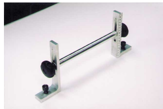
Bar for measuring press and lift with the foot
