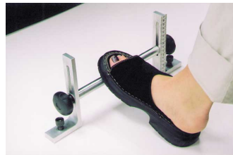
Measuring press strength on the bar
