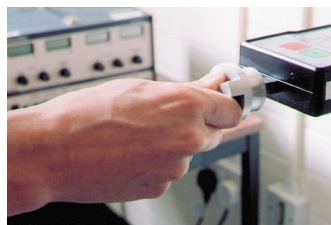
Measuring twist force on the push and turn knob
